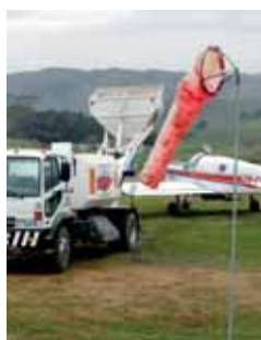
A windsock must be in place when a top-dressing plane is operating
