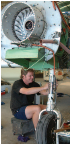
Paul Crimp carries out a check on the nose gear of a PT6-powered Fletcher
