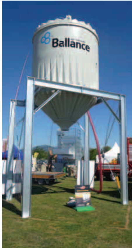
The silos destined for the West Coast have a unique design that eliminates product blockages by using angled cones to push and pull product through the spout
